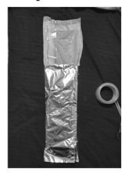
**Step Four:** after 3 wrappings cut the foil I folded the interior bag out over the foil to ensure it's completely insulated. Then bagged it again. Each exterior bag I taped the excess bag to itself to keep the foil layers
